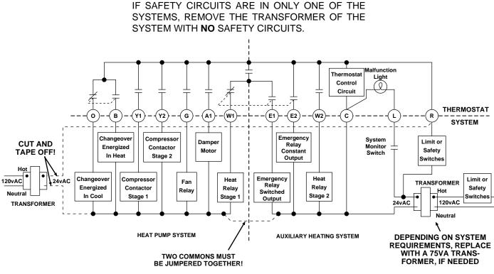
Figure 5. Typical wiring diagram for two-transformer system with NO safety circuits
